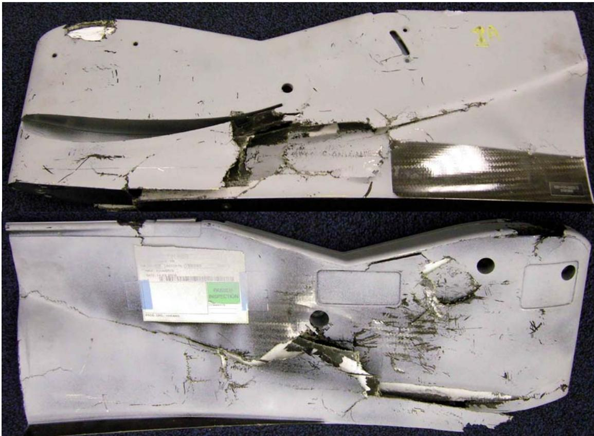
**Figure 2:** *Front and rear views of a Kevlar/carbon front wing endplate destroyed by instrumented impact testing and a “madman with a mallet”!*
