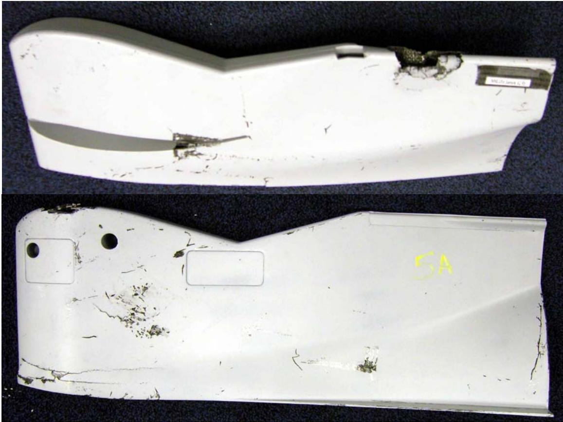
**Figure 3:** *Despite suffering the same fate as the specimen in Figure 2, the Innegra/Carbon front wing endplate remained intact and relatively unscathed.*
