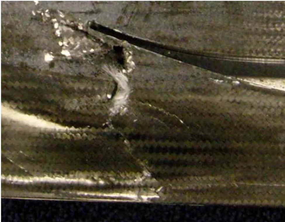
**Figure 4:** *When Innegra composite is damaged there is a tendency to tear and pull out fibres from the matrix rather than form sharp debris.*
